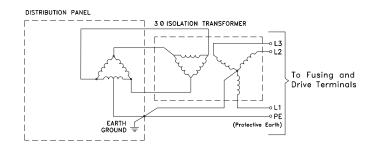
*Figure 7:* Three Phase Delta (with mid-phase GND) Distribution to a Three-Phase Delta/WYE Isolation Transformer
